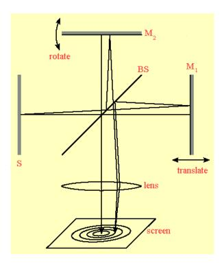
Figure 4: Basic schematic of the technology behind the Michelson Interferometer. [8]
