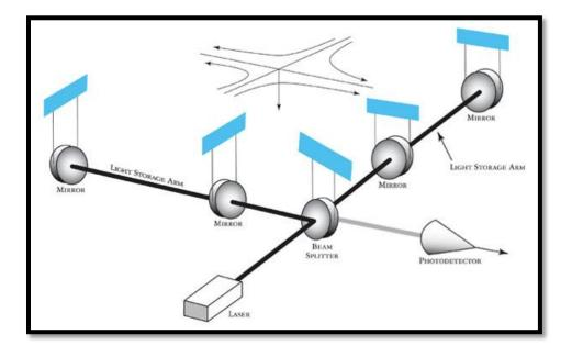
Figure 5: Diagram of LIGO's interferometers with an incoming gravitational wave depicted as arriving from directly above the detector. [9]
