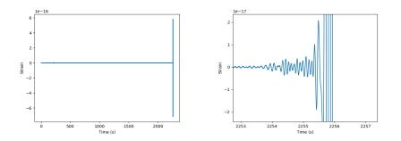
Figure 6: figure of LIGO strain data Figure 7: the zoomed in figure of the during Chile Earthquake spike in the previous figure
