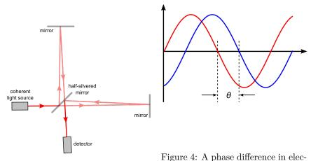
Figure 3: the basic structure of Michelson Interferometer <sup>[5]</sup>
