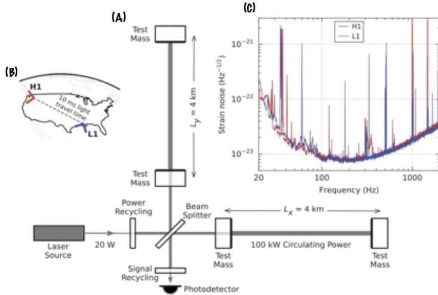
FIG. 1: (A) a simplified illustration of the Michelson Fabry-Perot Interferometer setup at LIGO. (B) relative positions and alignments of the two LIGO detectors in the United States: H1(Hanford, Washington) and L1(Livingston, Louisiana). (C) a strain sensitivity graph which represents the two detectors' individual strain sensitivities. [5]
