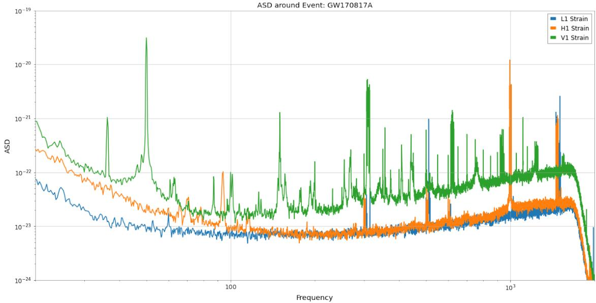
FIG. 6: The amplitude spectral density of L1, H1, and V1 for a time interval of 100 seconds near the proposed event GW170817A.
