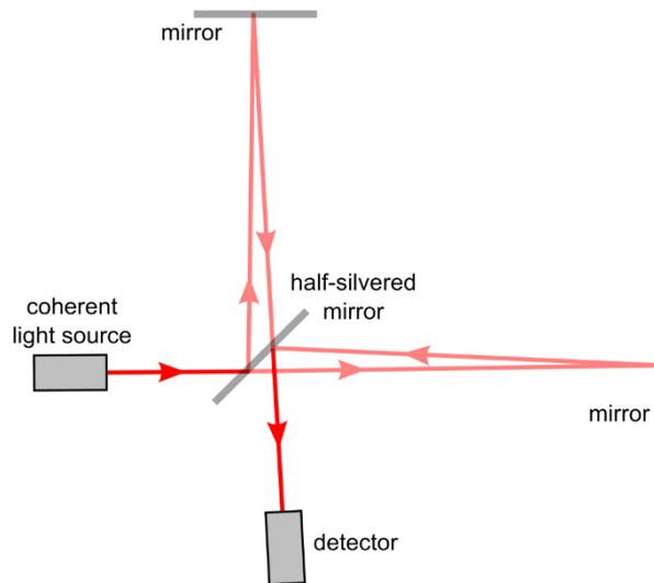
FIG. 1: The internal structure of a Michelson interferometer.
