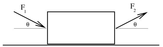
Let  $F_1$  and  $F_2$  be the force required to move the crate <u>at constant velocity</u> in the two cases. What can you say about the magnitudes of these two forces?
