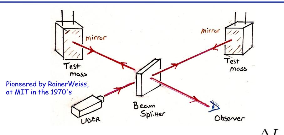
Measuring  $\Delta L$  in arms allows the measurement of the <u>strain</u> which is proportional to the gravitational wave amplitude
